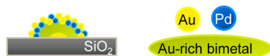
Figure 8. Schematic intersection of a PdAu particle on used PdAu/SiO 2 with an Au-enriched surface and a Pd-enriched subsurface layer.
